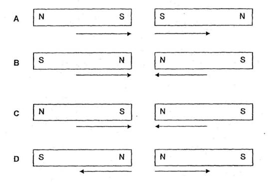
Which two of the diagrams (A, B, C and D) correctly show how the two bar magnets will interact when they are brought near each other?
